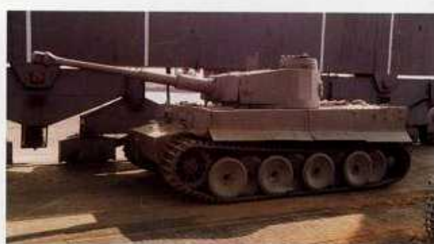
Armor protection on the hull sides of the Tiger I was about 2in thick. The rear engine hull plate and the bottom of the hull was roughly an inch thick. The horseshoe shaped turret of the Tiger I was 4in thick on the front and 3in thick on the sides and rear. The vehicle pictured is the Tiger I that used to be on display at the US Army Ordnance Museum and is now on a ten year loan to the German military museum system. The vehicle is seen here on its arrival in Germany on a dock where it was unloaded from the ship that delivered it. Thomas Anderson
