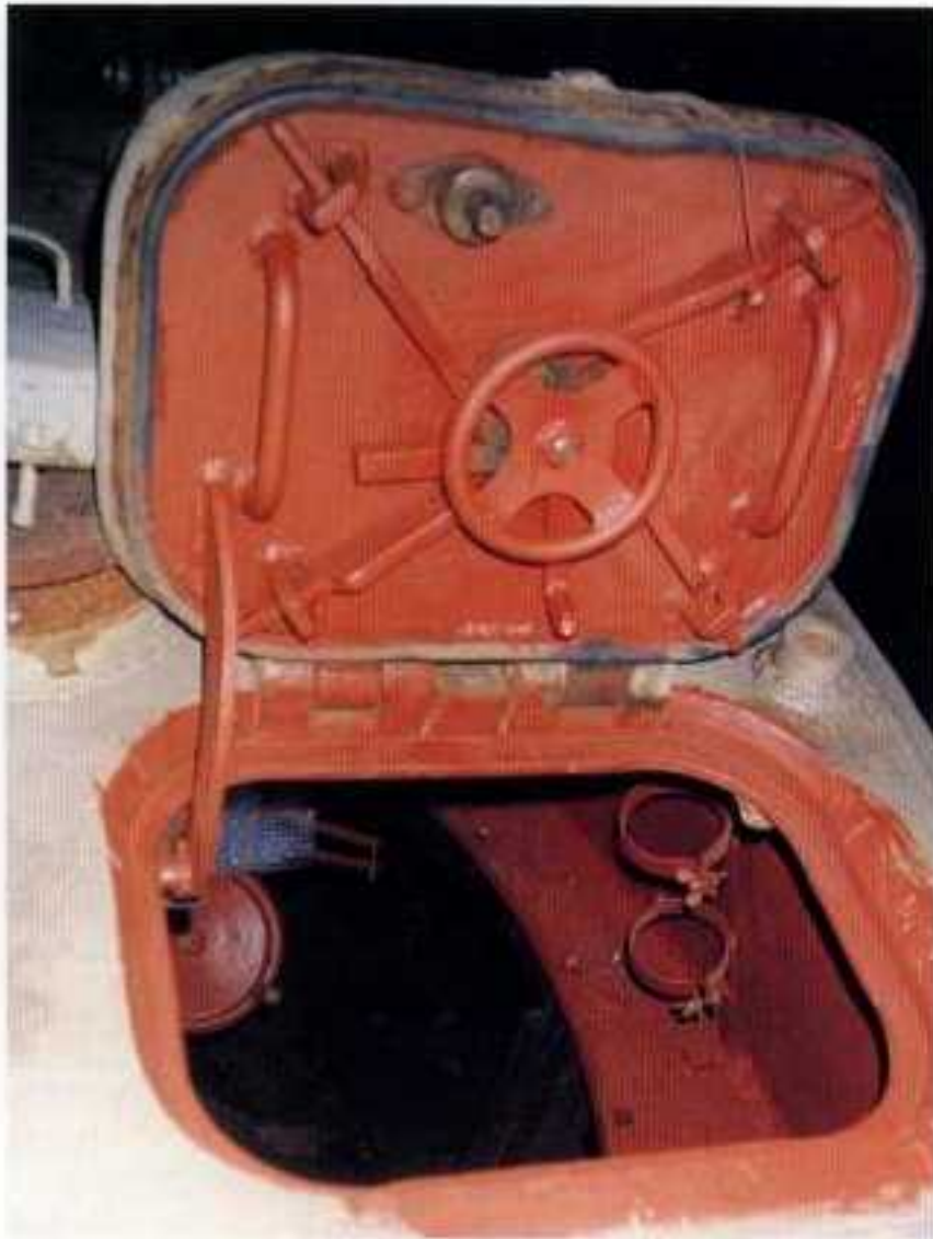
The loader's hatch on the Tiger I and Tiger IIs were identical. The hatch itself was rectangular in shape and was hinged at the front. This picture shows the loader's hatch of Tiger 332 at the Patton Museum. The interior of the vehicle has already been cleaned of rust and been given a primer coat. The upper portion of the hatch—as well as the uncovered ventilating fan seen to the upper left of the photo—shows the rust which had begun to eat away this historical vehicle. Patton Museum
