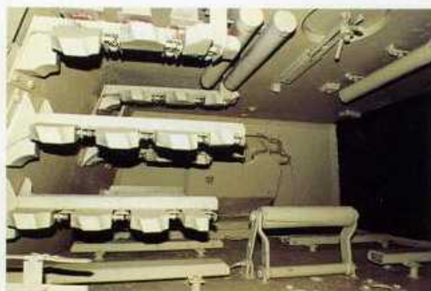
Unlike the Tiger I which had no main gun rounds stored in its turret, the Tiger II with its larger turret had space for up to twenty-two rounds when fitted with a Henschel turret and sixteen rounds when fitted with one of the fifty Porsche turrets. This interior photo of the Tiger II on display at the Patton Museum, shows the brackets for storing the main gun rounds in the rear of the turret. Located at the very rear of this Henschel turret can be seen the rear escape hatch. Seen at the bottom of the picture between the two sets of ammo racks is a wooden roller used to help the loader with placing the rounds into the gun's breech. Jacques Littlefield
