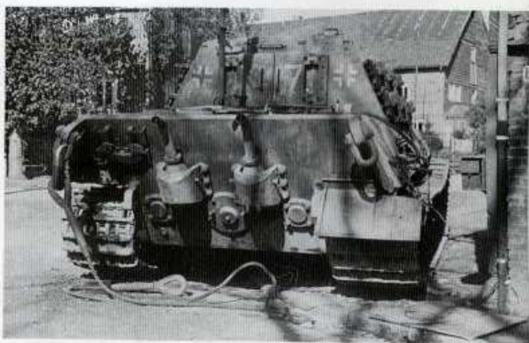
This US Army photo of an abandoned Jagdtiger shows the angled rear-engine deck shared with the Tiger II. Visible are the two mufflers and the vehicle's towing cable. On top of the rear engine deck is an monopod anti-aircraft mount for the fitting of an MG42 machine gun. Behind the machine gun mount, in the rear of the armored superstructure, can be seen the twin rear-access doors. These doors could be used as a means of loading the vehicle or as an escape hatch for the crew. Unlike a tank, the Jagdtiger's main gun was not traversable except for a few degrees on either side. To aim the main gun the entire tank had to be turned.
