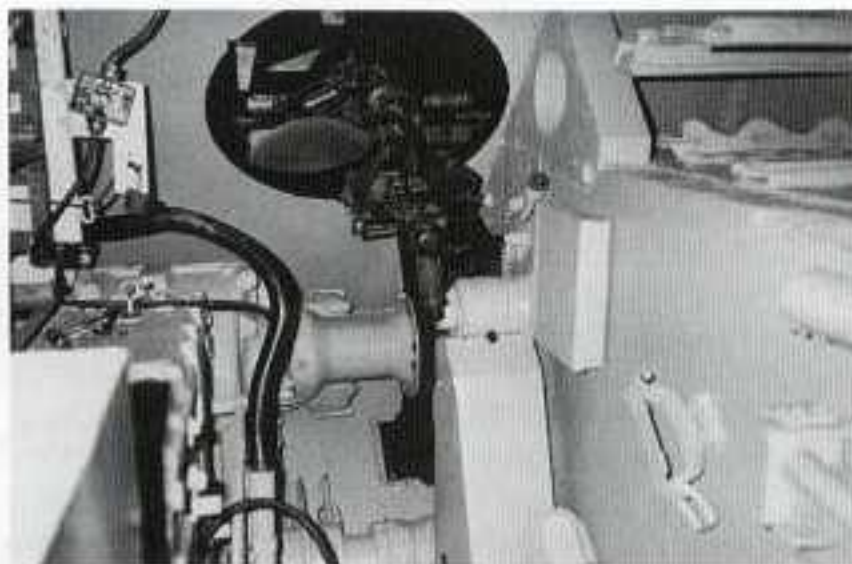
This interior close-up picture of the bow gunner's position on the Tiger II currently on display at the Patton Museum of Cavalry and Armor, shows the ball-mounting for a MG34 7.92mm machine gun. The machine gun and it's mount are shown in this photo. Jacques Littlefield
