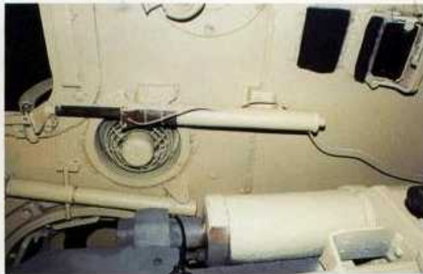
The loader hatches on both the Tiger I and Tiger IIs were spring assisted. This interior view of a Tiger II taken from the loader's position shows the spring piston and arm mounted on the inside of the turret roof. Located behind the spring piston and arm is the turret ventilating fan. On the far right of the picture is the loader periscope mount, with an overhead pad so the loader won't bump his head on the turret roof when looking through the periscope. Jacques Littlefield
