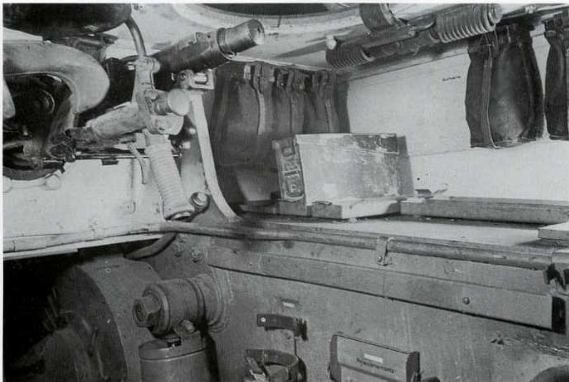
Taken inside of a Tiger I, this picture shows the hull-mounted 7.92mm machine gun as operated by the vehicle's bow gunner/radioman who was located in the front right corner of the hull. The machine gun itself is housed in a ball-mounting and controlled by a pistol grip which is visible in the center of
