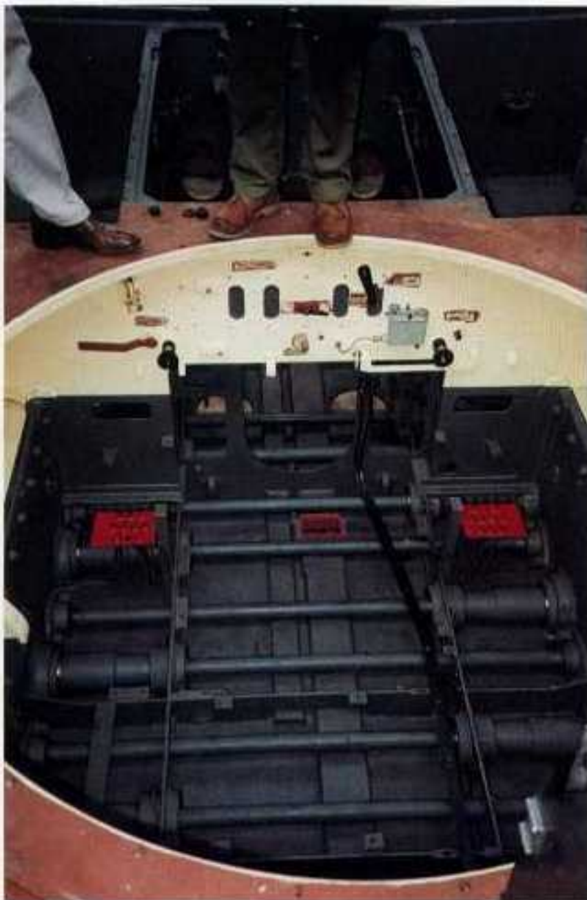
This picture is from the Tiger I located at the British Army Tank Museum, who's turret has been removed prior to rebuilding. The vehicle's empty engine compartment is located at the rear of the picture. The vehicle's drive train linkage has also been disconnected and removed. Seen on the bottom of the hull floor are the traversing torsion bars. Jacques Littlefield
