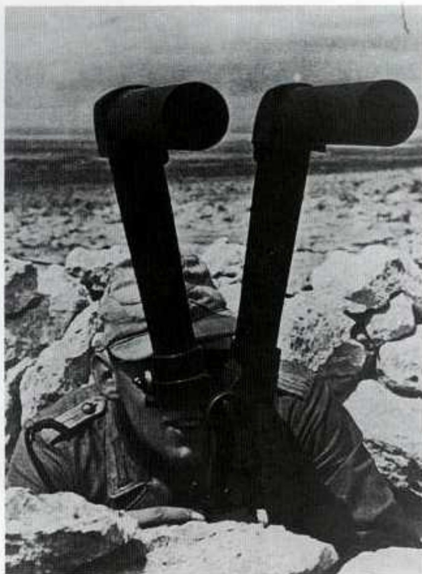
From a German wartime magazine comes this picture of a small scissors-type periscope being used by a member of General Rommel's famous Afrika Korps. This same device was also adapted to fit on the tank commander's cupola of the Tiger I. Used for observation, spotting, and for general conduct of fire, the binocular (two lens) construction increases the observer's stereoscopic (depth) perception. The periscope allowed a Tiger tank commander to keep his head under cover and still observe the fall of his main gun rounds.
