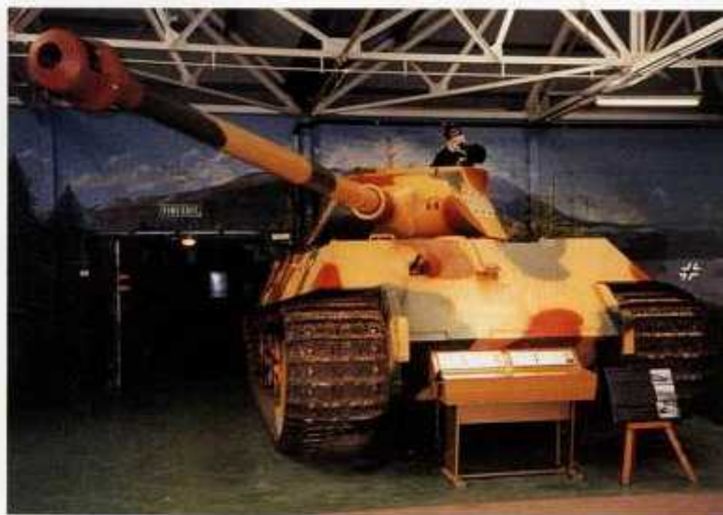
The Western Allies first encountered Tiger IIs in France in July 1944. Most of the Tiger IIs that fell into Allied hands during those initial encounters were fitted with the Porsche turrets, as is the vehicle pictured. The Tiger II's highly-sloped frontal armor was so similar in layout to that of the earlier Panther medium tank that in combat action, most Allied soldiers had a hard time telling them apart. This often led to the belief that the Germans were employing many more Tiger II's in France than there actually were. In actual numbers, German wartime reports show that there were never more than fifty Tiger IIs in France at one time. The Tiger II with a Porsche turret pictured is on display at the British Army Tank Museum. Bill Nahmens
