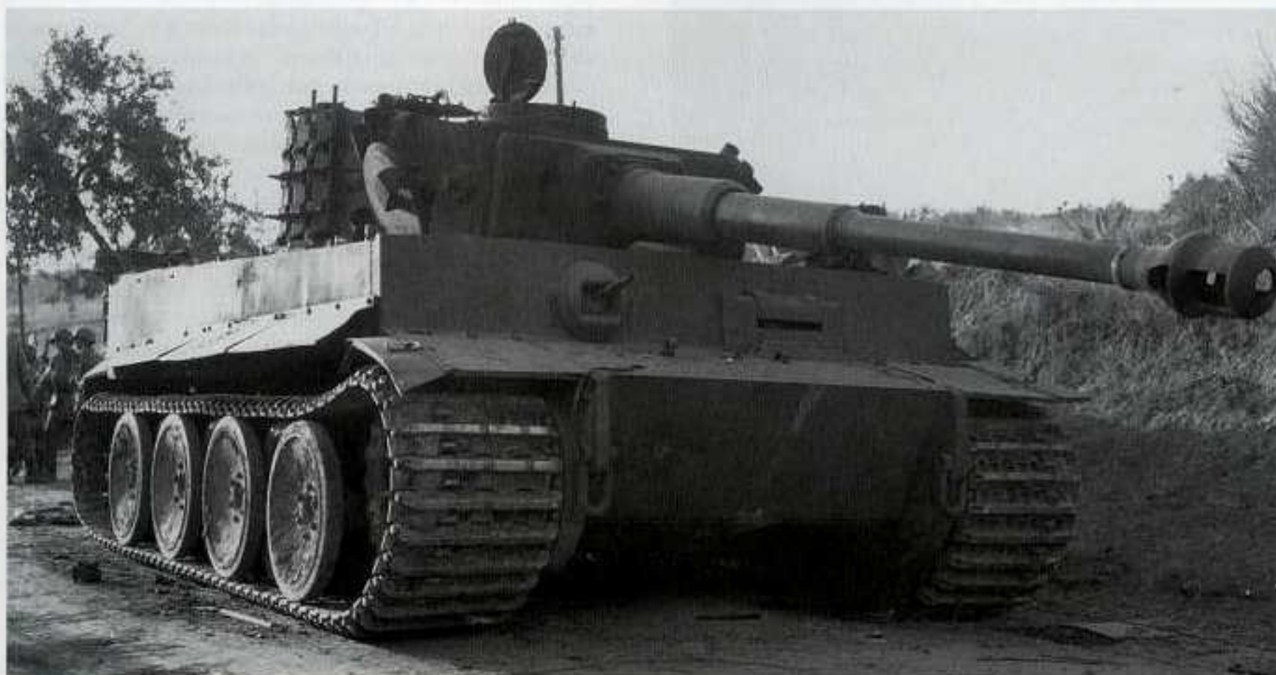
The very thick box-like hull armor of this early-model Tiger I can be seen in this photo of a captured vehicle in Italy. On the front superstructure hull plate can be seen both the hull-mounted 7.62mm machine gun and the driver's vision port
