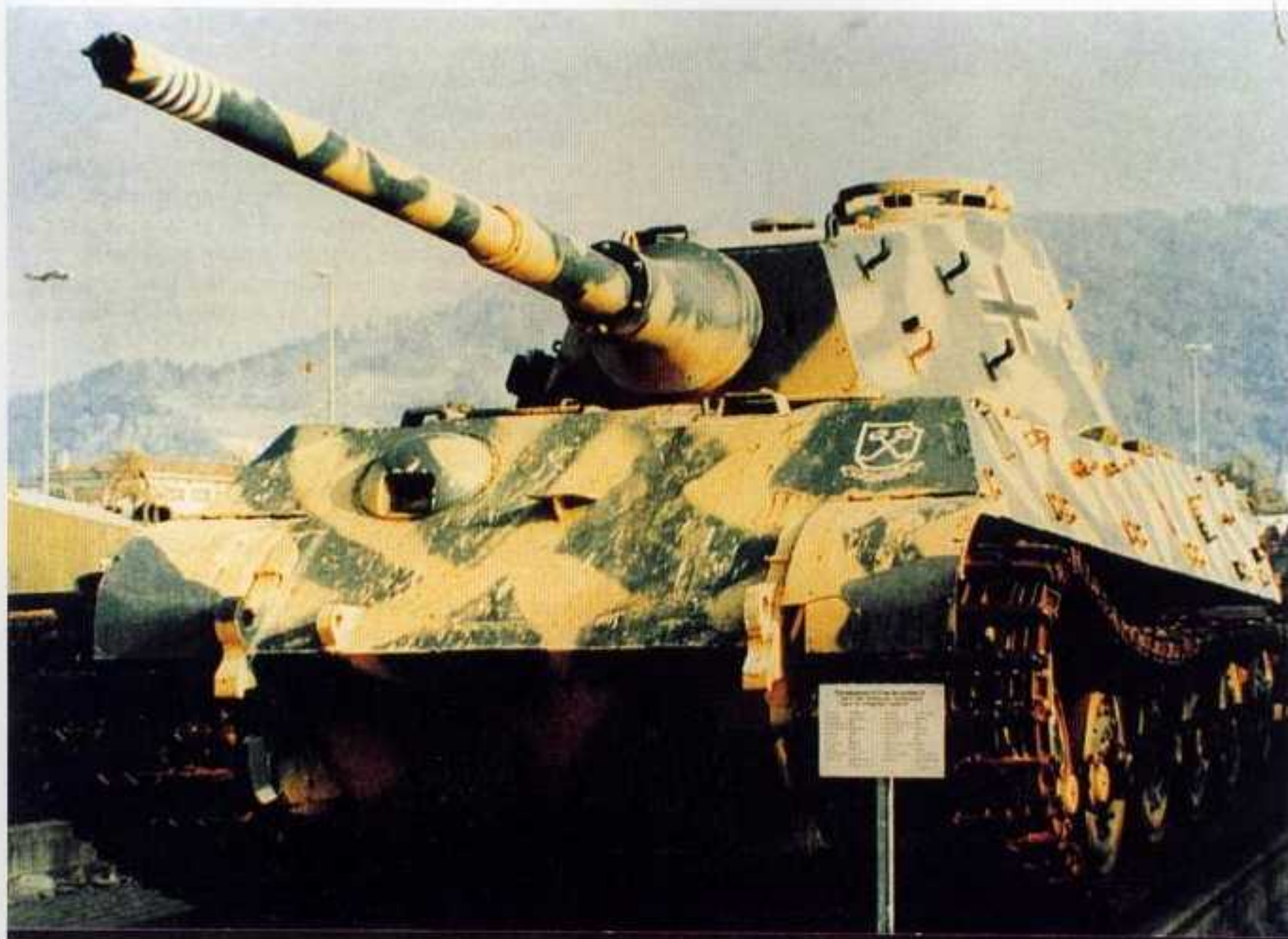
On display at the Swiss Army Technical Museum in Thurn, Switzerland, is a Tiger II fitted with an Henschel production turret. This particular vehicle is missing its muzzle brake. Protected by thick well-sloped frontal armor and armed with a
