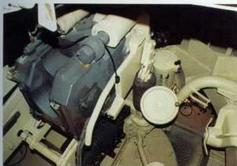
This turret-interior photo of the Tiger II belonging to the Patton Museum shows both the breech end of the KwK 43 gun and the loader's position. A breech mechanism is a mechanical opening and closing device located on the end of the barrel which provides for the entry and sealing of the ammunition in the weapon. On the other side of the breech is the folded-up seat and backrest of the tank commander. The gunner seat and controls would be located in front of the tank commander's position. Directly behind the main gun breech would be the ammunition racks for the main gun. Jacques Littlefield
