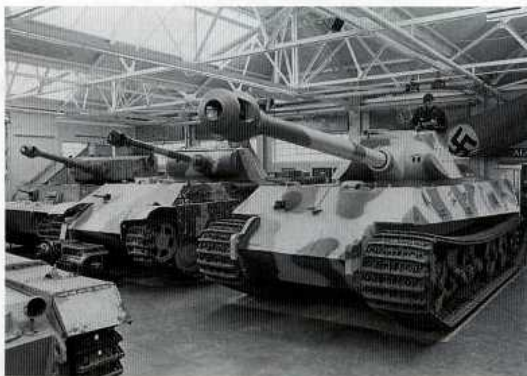
This photo—taken at the British Army Tank Museum, located in Southern England—shows the three best known German tanks of World War II. On the far left is the Tiger I with its box-like hull which first came off the production line in Sept. 1941. Next to the Tiger I is a Panther medium tank which came out in May 1942. The Panther was the first German tank to feature sloped armor in its design. The Tiger II prototype on the right of the Panther is fitted with the Porsche turret and clearly shows the influence of the Panther design. In combat, many Allied soldiers had a very hard time telling the difference between the two vehicles. The Tiger II reached the field in November 1944. British Tank Museum
