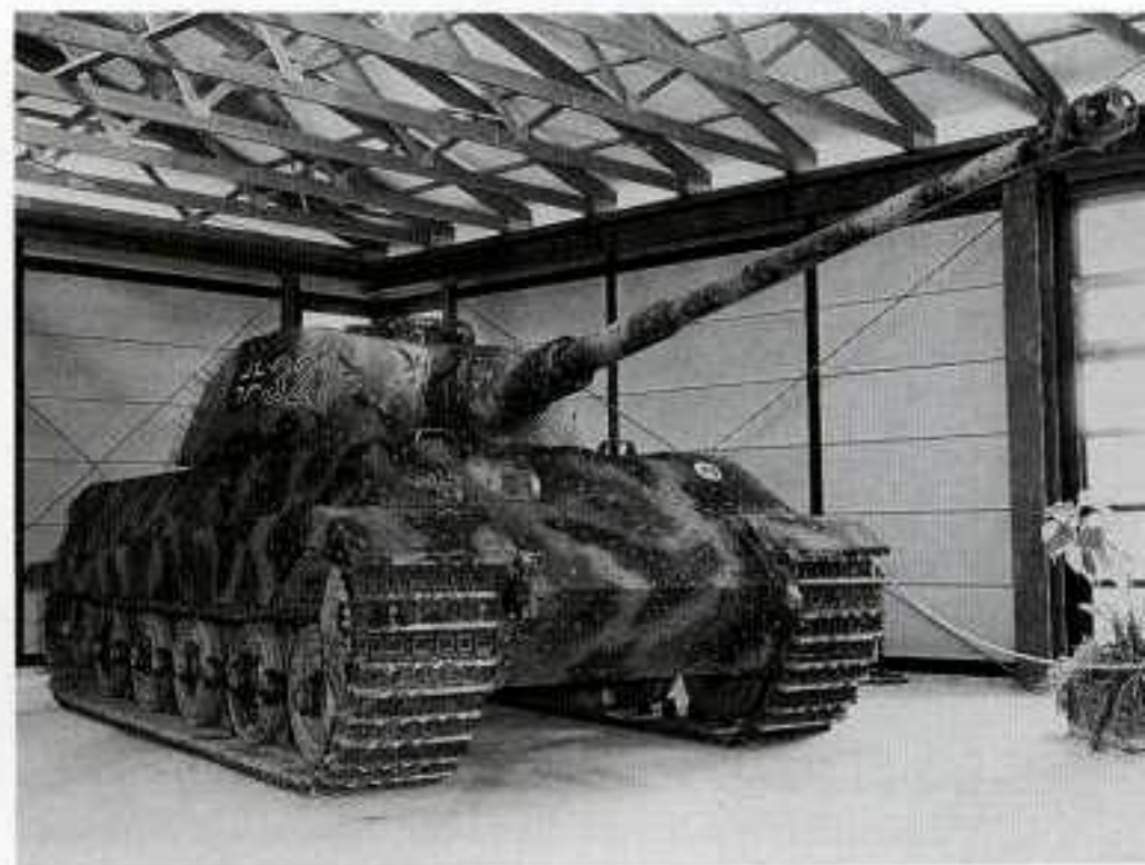
The Tiger II was armed with the final and most powerful version of the "88" family of guns, known as the KwK 43. This gun was 20ft 7in long. Like the KwK 36 version of the "88" mounted on the Tiger I, the KwK 43 as found on the Tiger II had a large double-baffle muzzle brake fitted. Some later production models of the Tiger II featured a slightly smaller version of the standard Tiger muzzle brake. The Tiger II pictured is currently on display at the German Army Tank Museum in Munster. German Army
