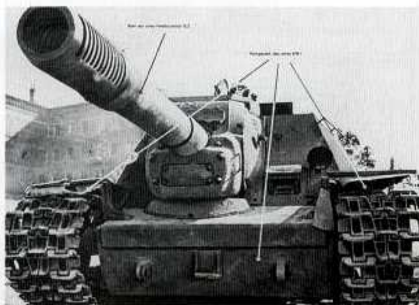
In response to the fielding of the Tiger I in early 1942, the Soviet military rushed into service as a stop-gap measure a specially-built tank destroyer armed with a fixed gun large enough to destroy or damage a Tiger tank with a single round. The official name for this vehicle was the SU-152. Armed with a ML-20 152mm gun-howitzer this vehicle first saw action against German Tiger Is during the large tank battles around Kursk in July 1942. During these battles the SU-152 destroyed at least a dozen Tiger Is. The photo of this massive vehicle comes from a German wartime manual. British Army Tank Museum
