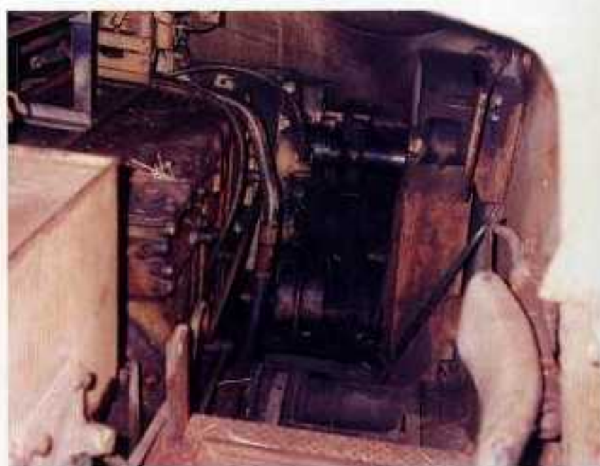
This picture, taken from inside the hull of Tiger 332, shows the bow gunner position. The bow gunner was also responsible for operating the vehicle's radio equipment—which is missing from this particular vehicle. When fitted, it was mounted to the left of the bow gunner on top of the gearbox. The leather pad that the bow gunner sat on is also missing from this vehicle. However, the bow gunner's fold-away backrest can be seen in the lower right hand corner of the picture. Where the radio operator's feet would be located, are components from the vehicle's final-drive gear housing. Patton Museum
